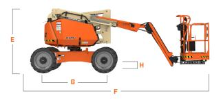
Platform Width 30-in / 0.76-m Platform Length 60-in / 1.22-m В. C. Machine Width 6-ft 4-in / 1.93-m ۵. 2-in / 5.08-cm Tailswing Machine Height 6-ft 7-in / 2-m Ε. Machine Length 18-ft 2-in / 5.52 m
