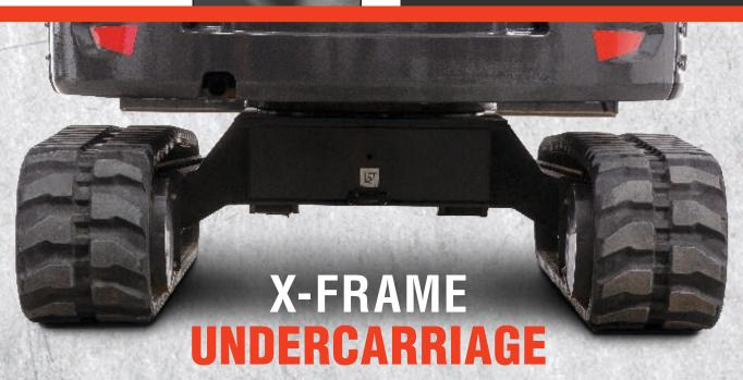
The X-frame design offers increased ground clearance that allows you to go through more. The design sheds debris to reduce your clean-up time as well.
