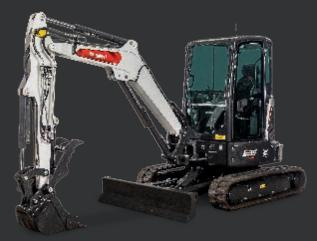
24.8 hp (18.5 kW) Standard, Long or Extendable Arm 121.2 in. (3077 mm) – 153.2 in. (3892 mm) Dig Depth
