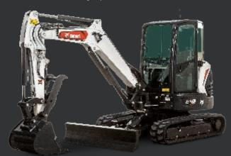
42.6 hp (31.4 kW) Standard, Long or Extendable Arm 124.5 in. (3163 mm) – 148.4 in. (3769 mm) Dig Depth
